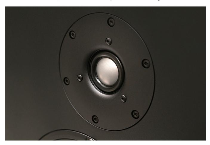
The tweeter, which Magico calls the MB30, is made by Scan-Speak and customized for the S5. Its 1" dome is made of beryllium, whose stiffness allows the dome's response to approach 40kHz without incident, whereas typical tweeters, with domes of aluminum or titanium tend to break up just above or even below 20kHz, at the theoretical upper limit of human hearing.
